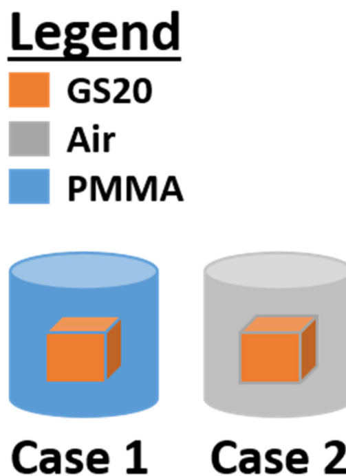
FIG. 2. Optical-ray-tracing simulation cases for a composite without air voids and for a composite with air voids. The color legend indicates the materials used for each case.
