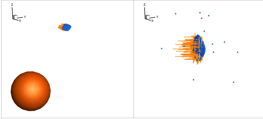
Figure 3. Left: a frame from the upcoming simulation of the deflection of asteroid headed towards Earth with an impulse applied to the asteroid (orange arrows). Right: a zoom on the impulse-asteroid interaction and resulting fragments.
