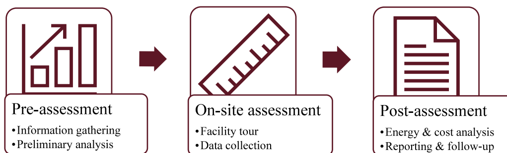
Fig. 8. Flow chart of industrial energy assessment procedure.
