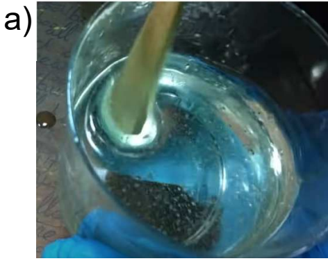
Epoxy Resin/Hardener Mixer (W:W/10:3)
