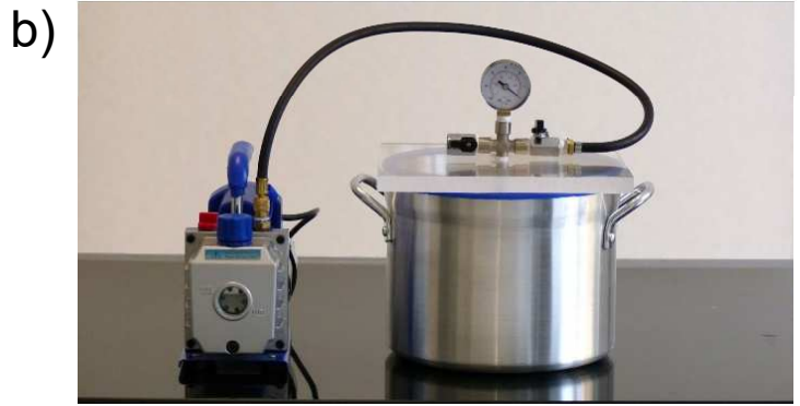
Degas: 20 minutes under vacuum. (Vacuum Level: 25.5" Hg)
