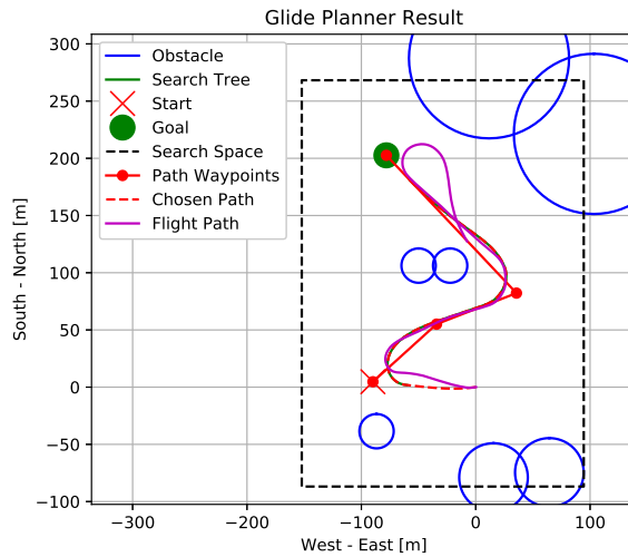
Fig. 15 The plot shows the full planning result from one of the path plans, along with the X-Y position of the flight path.
