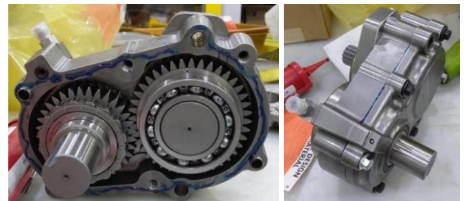
FIGURE 17: ASSEMBLED PTO GEARBOX
