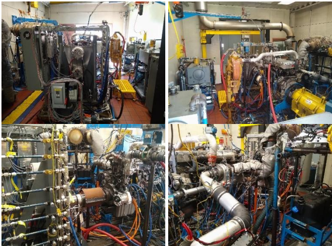
FIGURE 11: FINAL H2D2 FULL HYBRID SYSTEM VALIDATION TEST INSTALLATION
