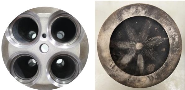
FIGURE 15: TBC CYLINDER HEAD AND PISTONS SUCCESSFULLY MANUFACTURED
