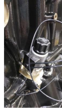
FIGURE 16: SOLENOID INSTALLED INTO ENGINE BLOCK
