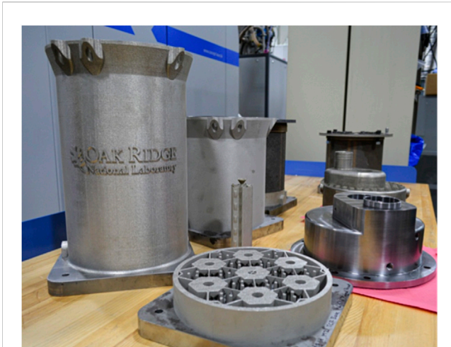
FIGURE 6 3D printed components for the prototype reactor. Credit: B. Cramer, ORNL (Oak Ridge developing 3D-printed nuclear reactor core, 2020).
