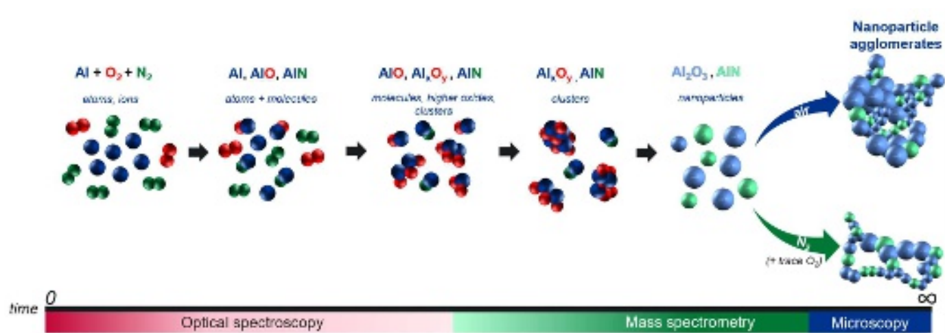
FIG. 11. Schematic summarizing the evolution of plasma species in laser ablation plumes to NP and NP agglomerate formation for air and \text{N}_2 (with trace \text{O}_2 ) environments.
