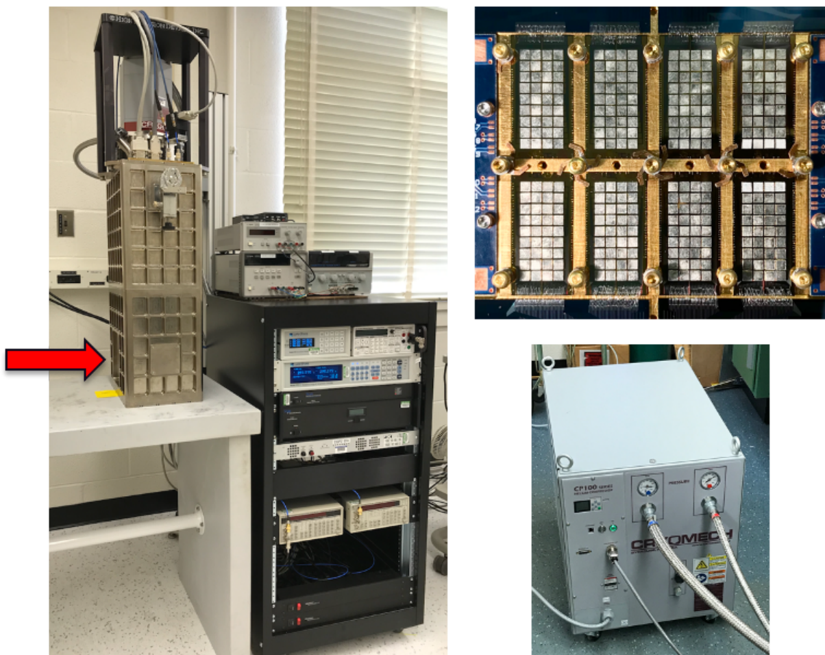
Figure 1: The compact SOFIA microcalorimeter spectrometer consists of a cryostat (left), 256-pixel multiplexed transition-edge sensor microcalorimeter array (top right) and an air-cooled compressor (bottom right). Items to be measured are placed next to the cryostat in front of the side-looking window (indicated by red arrow), or the instrument can be moved next to a glove box or hot cell port.
