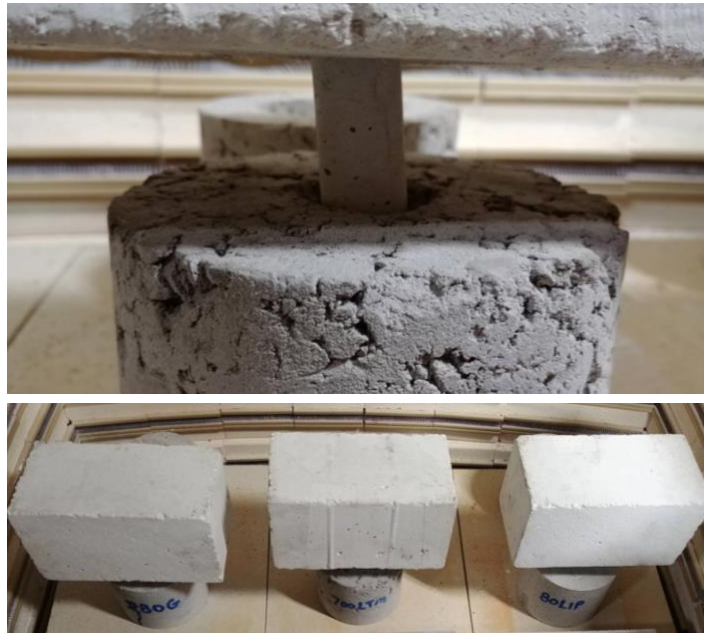
Figure 8. Compatibility testing with silica particles in crucible under a 140 kPa compressive load, which is similar in magnitude to that expected during operation [5].
