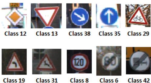
Fig. 18: Top 5 most (upper) and least resilient (lower) traffic signs and their GTSRB classes to bit-flips in the first convolutional layer.
