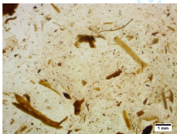
Figure 2: Optical image of solid particles in a diluted, untreated (control) corn stover slurry.
