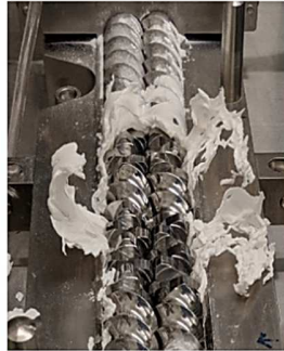
Figure 8: Examples of failure modes observed during the transfer from batch to continuous granulation
