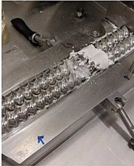
Figure 8: Examples of failure modes observed during the transfer from batch to continuous granulation
