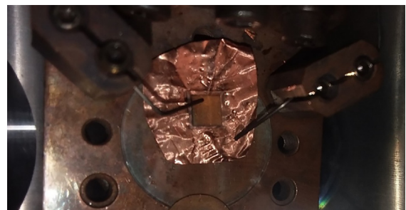
FIG. 1. Diamond detector mounted to the cold finger of the Janis VPF-800 cryostat.
