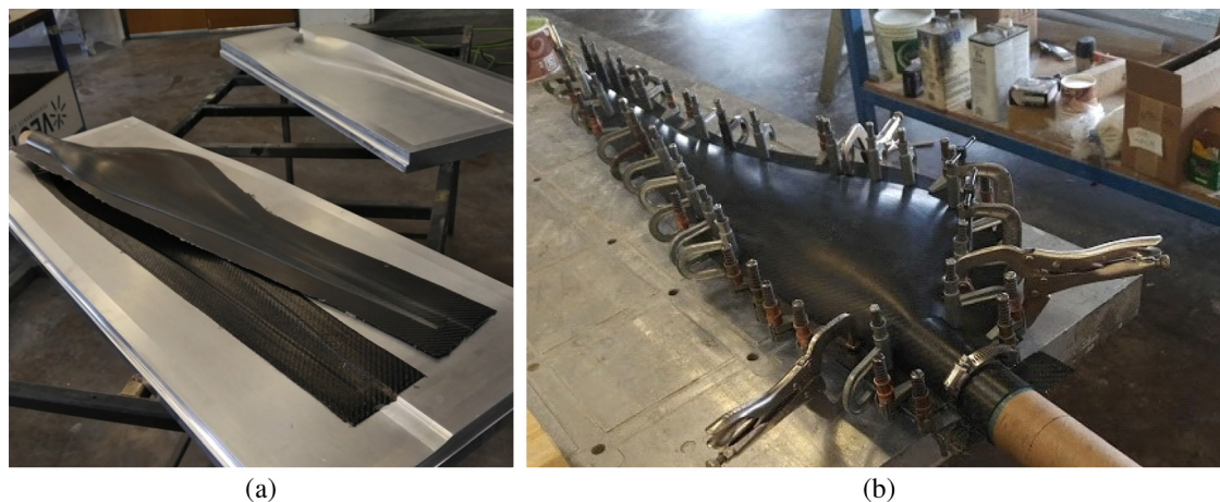
FIG. 3. Blade fabrication details: (a) aluminum molds with the resulting blade surfaces and (b) bonding of the blade surfaces.
