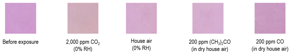
Fig. 4. PSP-ED/ZIF-8 profiles before target gas exposure; exposed to 2,000 ppm carbon dioxide (dry); dry house air; 200 ppm acetone (in dry air); and 200 ppm carbon dioxide (in dry air).
