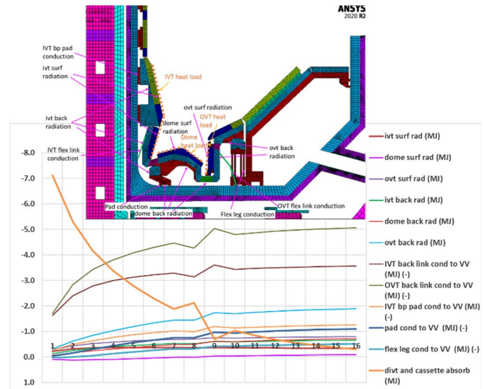
Fig. 9. Heat flow in the divertor-cassette region, by integrating power with respect to time.
