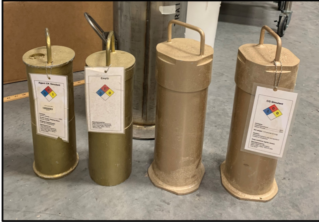
Figure 2: Mock 4.2-inch mortar casings used to contain the CK (left most) and CG (right most) simulants. Identical empty containers (center) were also used in the overpacked measurements to examine the spectral component arising from the vermiculite and munition casing (see text for details).
