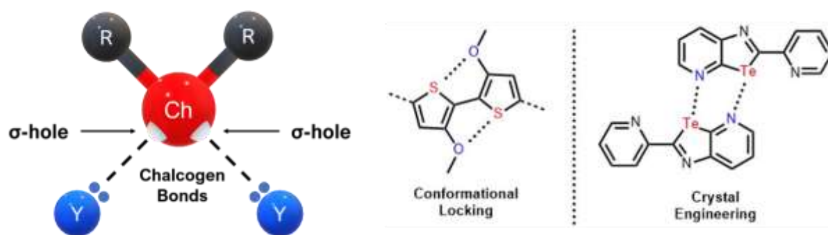
Figure 8. Schematic representation of chalcogen bonding interactions (left) employed in conformational locking strategies and crystal engineering (right).
