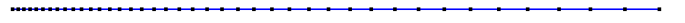
Figure 3: 1d mesh used to compute global thermo-mechanical RPV response. Second-order elements were used, and all nodes, including mid-edge nodes are shown.
