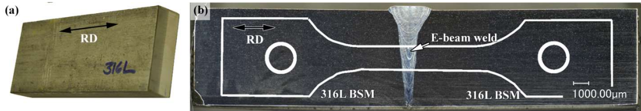
97 98 Figure 1. (a) The as-received 316L material and (b) a sample of 316L welded using e-beam welding. RD 99 represents the rolling direction of the as-received material. A tensile bar with close to typical dimensions 100 of a SS-3 type specimen is also drawn on the welded block. 101
