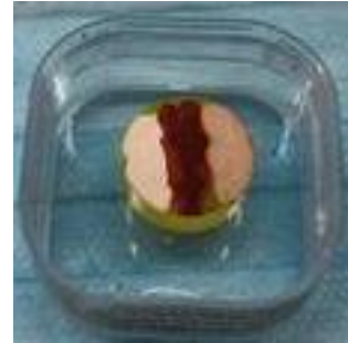
Fig. 2. A GYGAG(Ce) scintillator with three temperature sensitive paints was used to determine the maximum temperature at each of the fluxes used in the electron irradiations.
