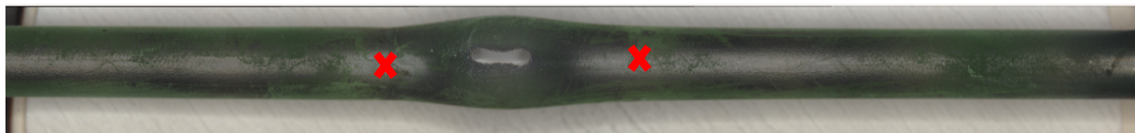
Figure 5. Post LOCA image of a Cr-coated Zircaloy 4 tube sampled with X's marking the location of thermocouples
