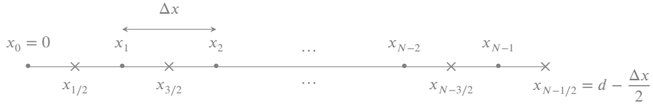
Figure 1: Staggered grid representing (x_i)_{0 \leq i \leq N-1} \in \mathbb{R}^N and (x_{i+1/2})_{0 \leq i \leq N-1} \in \mathbb{R}^N .
