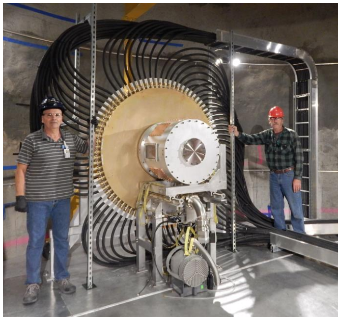
Fig. 1. MJOLNIR DPF in 1 MJ stored energy configuration.
