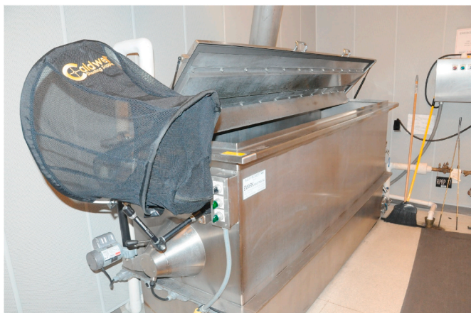
Fig. 4. Water tank used to collect bullets in groups of 50. An enclosure net was used to catch expended cartridge cases (Caldwell Shooting Supplies, Columbia, MO).
