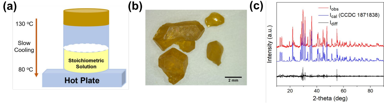
Figure 1. (a) A schematic illustration of the crystal growth process. (b) Photographs of the \text{Rb}_4\text{Ag}_2\text{BiBr}_9 SCs. (c) The obtained SCs do not have any impurity inclusions as judged by the comparison of the measured and calculated PXRD patterns of a crushed polycrystalline powder sample of \text{Rb}_4\text{Ag}_2\text{BiBr}_9 .
