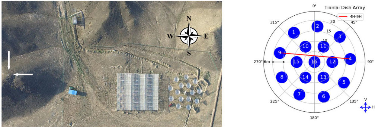
Figure 1. Left: A top view photograph of the Tianlai arrays, which consist of the dish array and the cylinder array. The photo was taken with a drone at a height of 280 m above the ground. The arrays saw first light in 2016. The position of the calibration noise source is indicated by the white arrows on the left. Right: A schematic diagram of the Tianlai dish array. The dishes are arranged in two concentric circles of radius 8.8 m and 17.6 m around a central dish. The dishes have dual-linear polarization feed antennas with one axis oriented parallel to the altitude axis (horizontal, H, parallel to the ground, or E–W in the figure) and the other orthogonal to that axis (vertical, V, N–S in the figure). For example, the red line shows one of the baselines that is the H polarization of dish 4 correlated with the H polarization of dish 9: [4H 9H]. The above image is reproduced from Wu et al. (2021).
