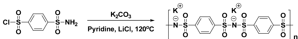
Scheme 13: Synthesis of an anionic polyarylsulfonimide, the first reported anionic ionene.
