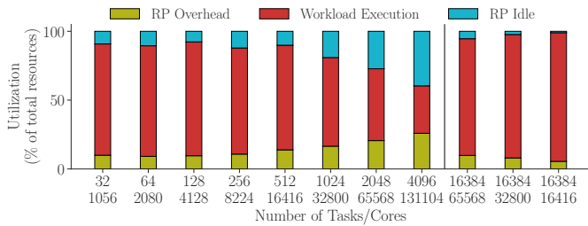
Fig. 7. Resource utilization (RU) of RADICAL-Pilot. First 8 bars: Experiment 1; Middle 3 bars: Experiment 2; Last 4 bars: Experiment 3.
