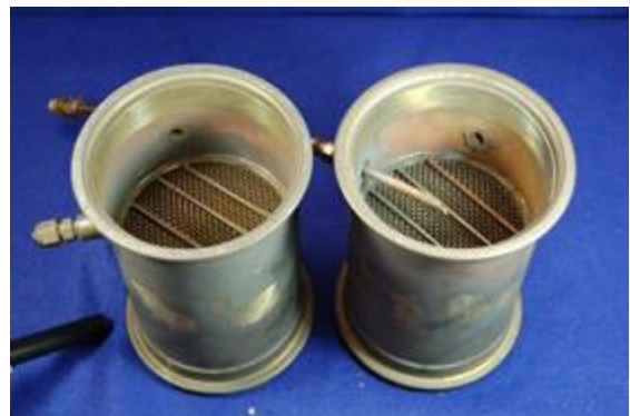
Figure 21. Photograph of the Microlith®-based reforming catalyst cylinders after approximately 100 hours of testing.
