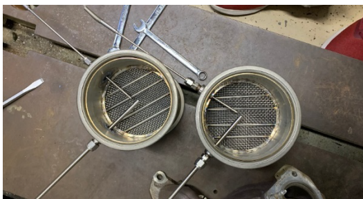
Figure 3. Picture of the Microlith ® reforming sections, developed by PCI, prior to installation in the engine. Also seen in the photograph are the thermocouples and gas sampling probes located at the catalyst-out position.
