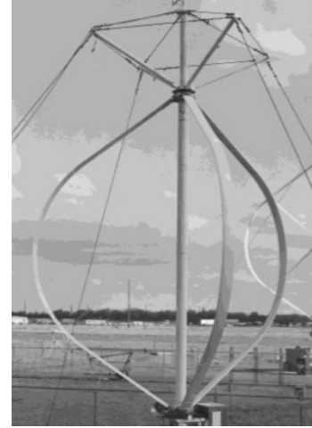
Fig. 2 SNL 5m three-bladed turbine showing troposkein shape.
