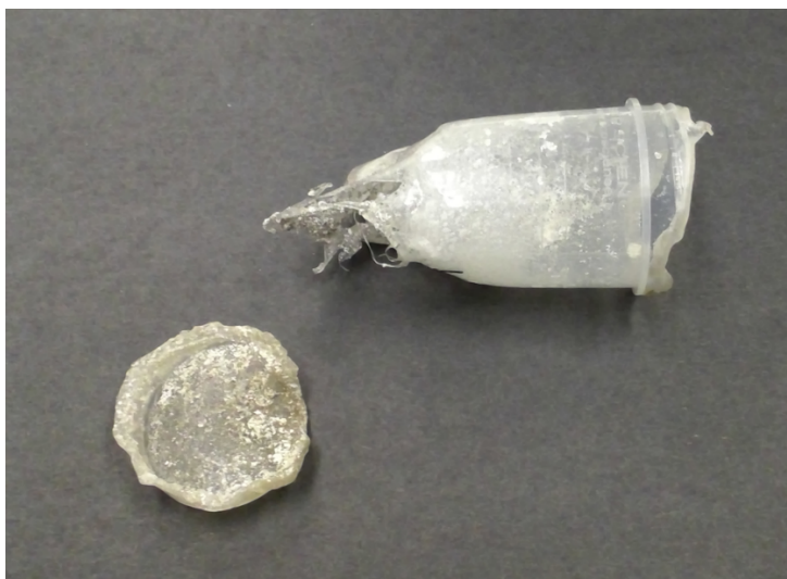
Figure 2: Post-accident photo of the tube containing lithium silicide fire.
