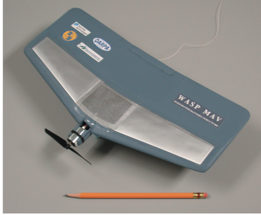
Figure 10: Darpa Wasp UAS with integrated Li-ion cells [88].
