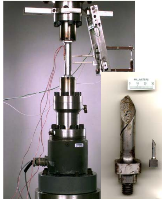
Fig. 1. SNTT configuration (left) and sample miniaturization for A533B steel (right).
