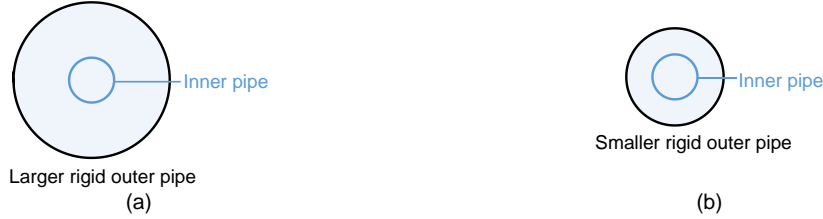
Figure 5. Two pairs of fluid-filled concentric pipes, including identical flexible inner pipes and rigid outer pipes with different radii: (a) larger outer pipe; (b) smaller outer pipe
