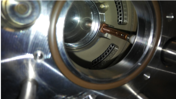
Figure 3: Top panel: A photo of the components at the downstream end of the Proton Detector. The field cage (center) is terminated in the gating grid (threaded through the green ring). The two copper rings are responsible for the drift field between the gating grid and the MICROME GAS (not in the picture). Four gas inlets and a rough pumping line surround the end of the tube. A feed-throughs port for the field cage ground and the gating grid is at the top. Bottom panel: A photo of the components at the upstream end of the Proton Detector. The aluminized mylar window reflects the 20 kV SHV feed-through. A copper finger connects the perforated cathode to the feed-through. The Kapton™ window is removed to allow the photo.
