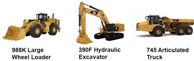
Figure 3. The three key machine applications selected for the baseline. All three are powered today by a Cat® C18 ACERT™ diesel engine.
