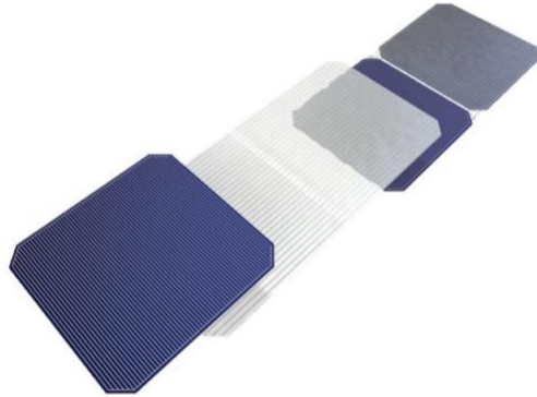
Fig. 1. Schematic of alignment of multiwire foils on cells prior to lamination [9]. The interconnects are formed during lamination due to the low melting point of the solder, reducing thermal stresses to the cell.
