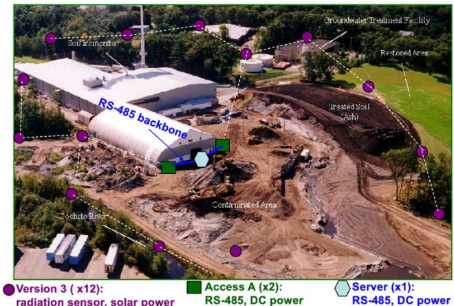
Fig. 30. Proposed deployment of integrated sensor system in an outdoor perimeter sensing and security location.
