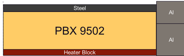
FIGURE 1. 2D axisymmetric representation of the experiment geometry. The PBX 9502 slab was 6” diameter, 1.5” thick.
