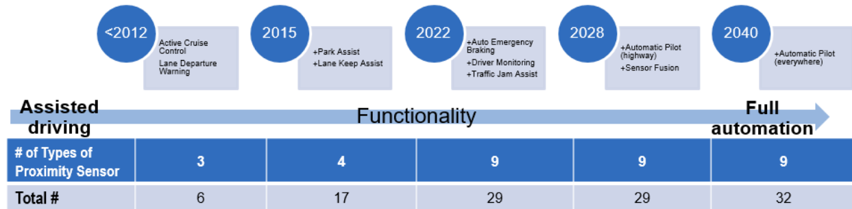
113 114 Figure 2: Advance Driver Assistance Systems (ADAS) and the projected increase in number of 115 sensors per vehicle (adapted from [20])
