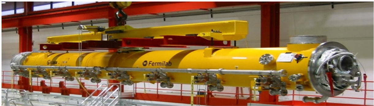
Figure 1. The 1.3GHz LCLS-II 12.2-meter-long SRF cryomodule made by Fermilab.
