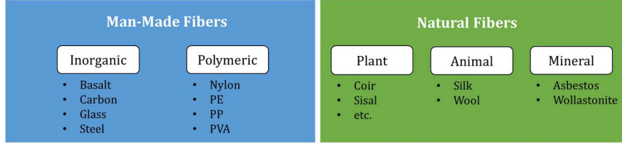
Fig. 2. Classification of fibers commonly used in cementitious materials.
