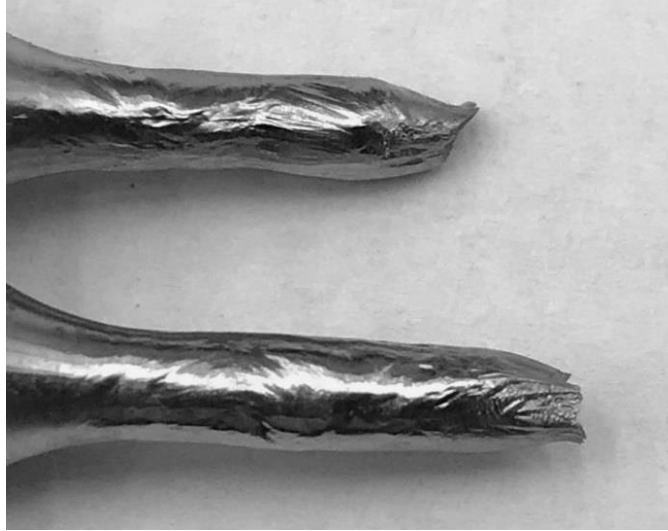
Figure 12: Photograph of a failed EBAM-W tensile bar showing the effects of large grains creating a lumpy surface throughout the entire gage length
