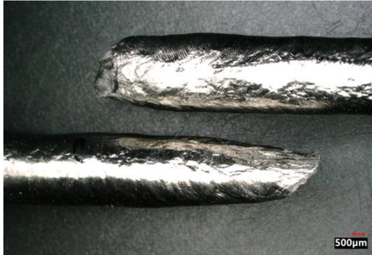
Figure 9: Photograph of a failed WAAM tensile bar showing the effects of large grains creating a dimpled surface in the gage length and at the necked region on the sample.
