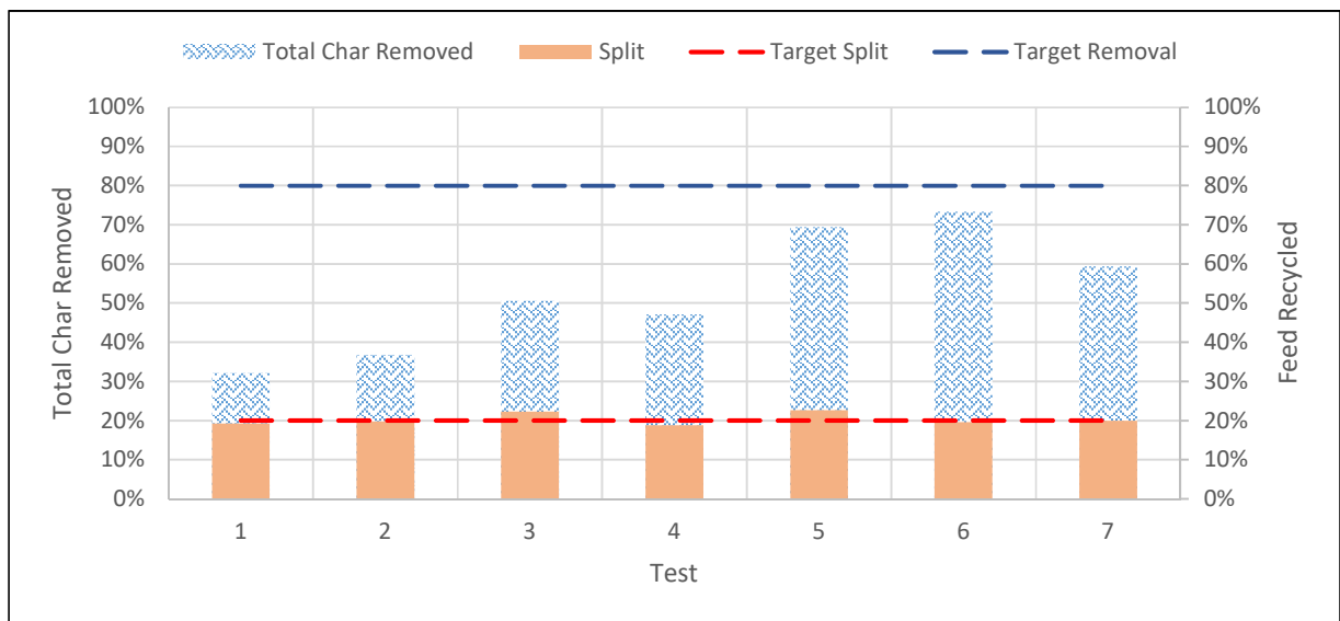
Figure 8. Cold flow LCS tests of 170 μm Ilmenite at different bed heights and solid feed rates. Bed velocity during all tests 1 U_{mf} equivalent with AB fluidization regime
