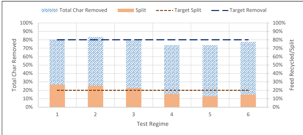
382 383 Figure 11. Hot flow test results at 800°C with 210 \mu\text{m} Ilmenite (1 - 4) and 170 \mu\text{m} Ilmenite (5 - 6) 384
