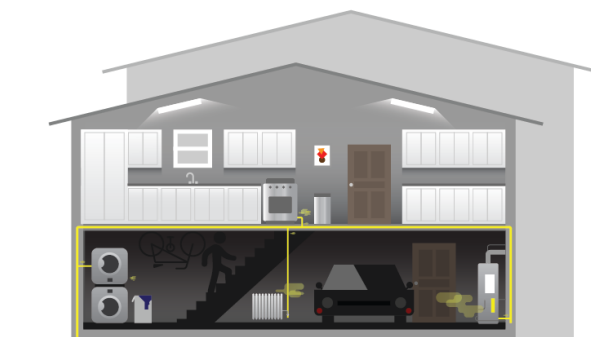
Figure 5. Schematic of appliances and devices within a residence that contribute to CH 4 emissions, which can be measured from individual components or as whole-house emissions 1, 59 .
