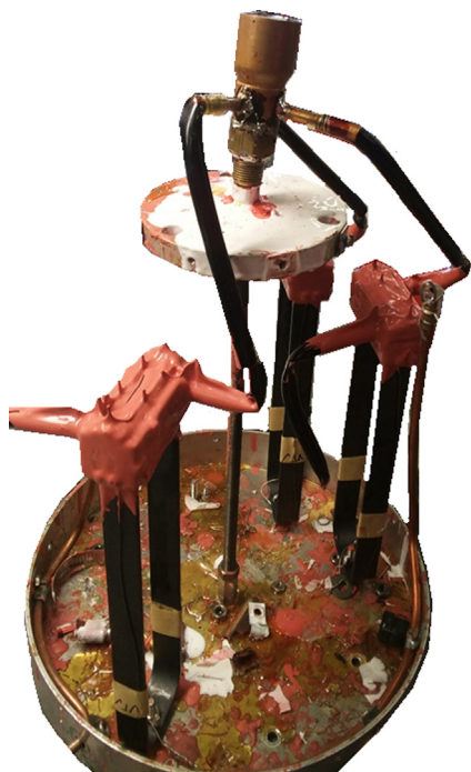
Fig. 3. TPI sample vacuum impregnation fixture carrying two samples.
