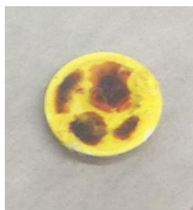
Figure S11. Photo of a piece of PIN-coated LATP after being cycled for 150 cycles in a Li || PIN-LATP || S/C cell.
