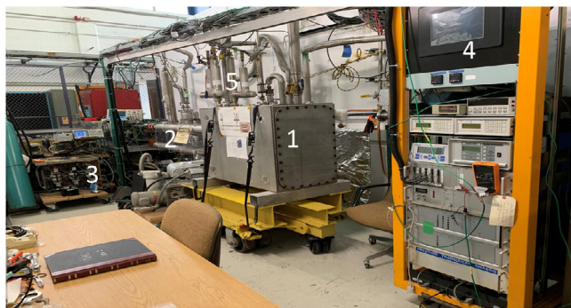
Fig. 6. View of the HTS test magnet setup: 1 – magnet, 2 – current leads, 3 – power supply, 4 – cryogenics and power supply controls, 5 – cryogenics support.
